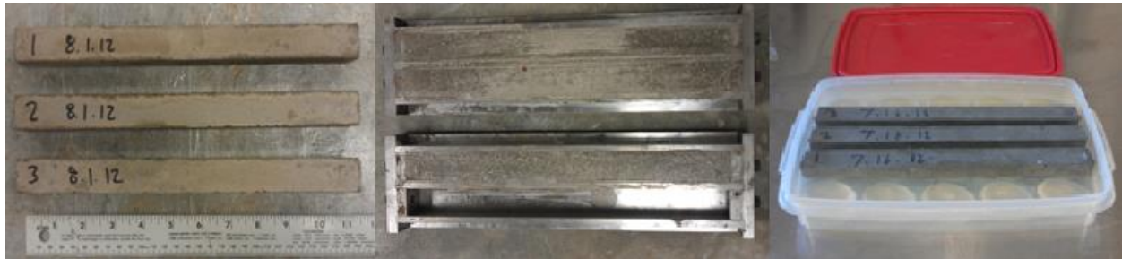
Figure 2.2 – AMBT left to right specimens. Specimens in molds, and specimens in alkali bath (Deschenes 2014)
